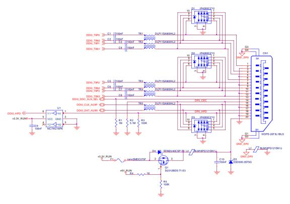
The example schematics in the following page, instead, shows the implementation (using DDI interface #2, but any DDI can be used for this purpose) of a double connector DP++ and HDMI, managed using a DisplayPort 1:2 Switch with Integrated TMDS Translator, which provides to TMDS voltage level shifter for HDMI/DVi connection.
